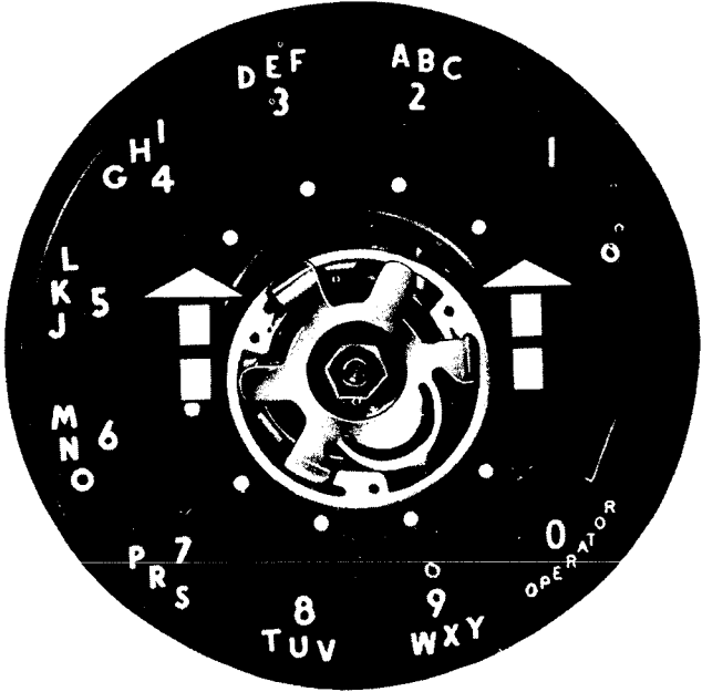
Fig. 8 — Lock Ring in Extreme Forward Position for Removal
