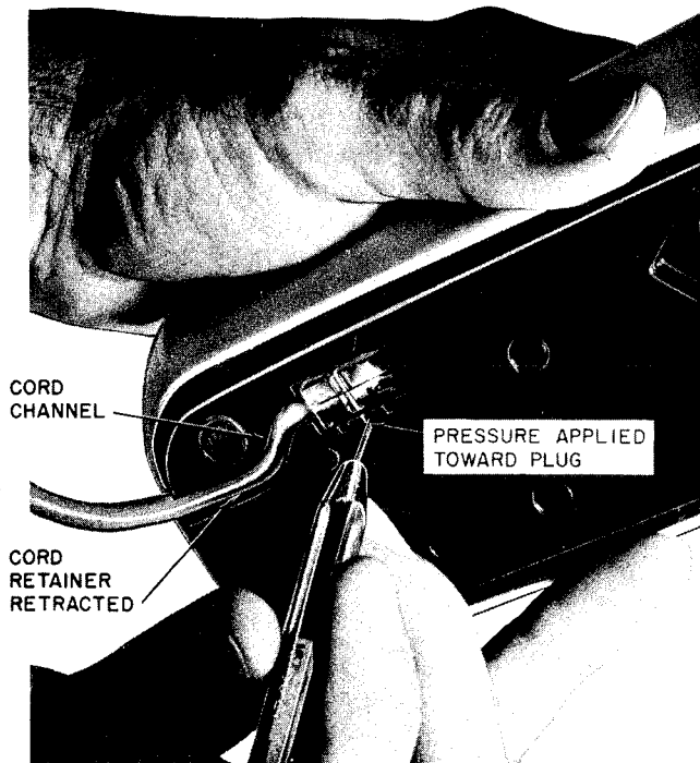
Fig. 12—Removing Mounting Cord From AD1 telephone Base
