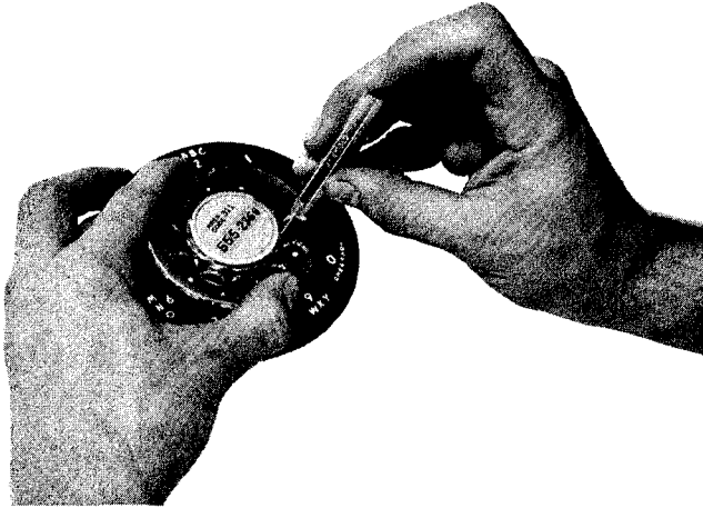
Fig. 4 — Removing Plastic Fingerwheel
