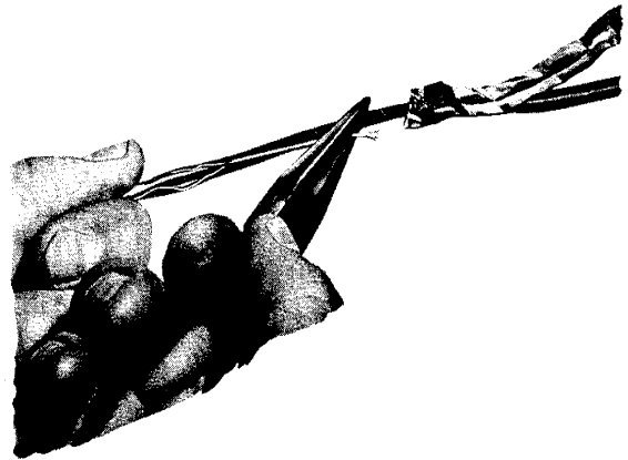
Fig. 2 — Slitting Inner Jacket, Using Slitting Cord
